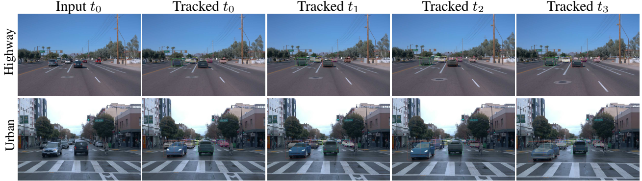
Figure 3. Without changing the model or training on the dataset, our proposed method can generalize well to the Waymo Open Driving Dataset [37]. Similar to Fig 2, from left to right, we show (i) observed images from diverse scenes from the dataset at timestep k = 0 ; (ii) an overlay of the closest generated object and predicted 3D bounding boxes at timestep k = 0, 1, 2 and 3. The color of the bounding boxes for each object corresponds to the predicted tracklet ID. Our method does not lose any tracks even on a different unseen dataset in diverse scenes, validating that the approach generalizes.
